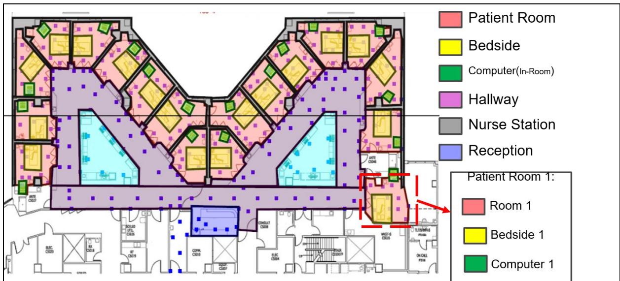
Figure 2: The layout of ICU with NFER calibration points
